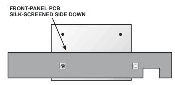
Figure 4. Preparing Front Panel PCB to Install Light Bar.
