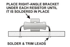
Figure 15. Spacing the 1-watt and 3-watt Resistors above the PCB.
