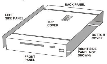
Figure 1. XV Transverter Modular Cabinet Parts.
