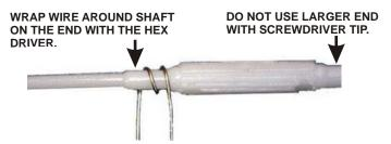
Figure 34. Winding L10 on the Alignment Tool.
