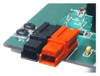
Figure 28. Orienting J7 on the RF PCB.
