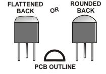
Figure 7. Transistor Orientation Guide.
