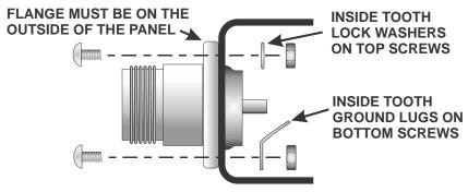
Figure 30. Mounting the Antenna Connector J1 on the Back Panel.
