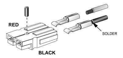
Figure 47. Power Cable Connector Assembly.
