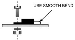
Figure 19. Installing Voltage Regulator U4.
