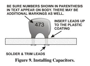
Install capacitor C4, .001  $\mu$ F (102) on the *back* side of the PCB (the side that is *not* silk-screened).
