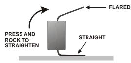
Figure 44. Straightening IC Pins.
