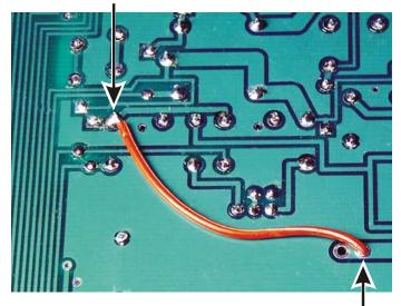
**RED FAN WIRE FROM TOP OF PCB Figure 38. Fan Wire Routing on Bottom of PCB.**
