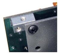
Figure 41. Bottom Cover Attached to a 2-D Fastener.
