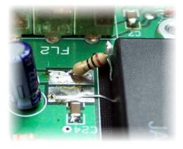
Figure 43. 10 Ohm Resistor Installed on the RF Power Module.
