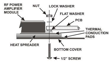
Figure 42. RF Amplifier Module Mounting Hardware.
