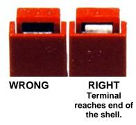
Figure 27. Verify Contact is Fully Inserted.
