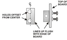
Figure 31. 2-D Fasteners.
